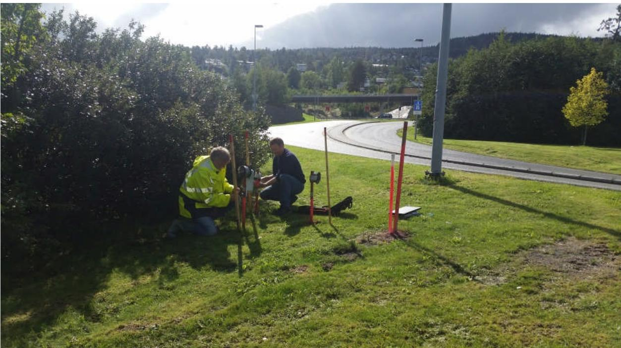
**Fig. 1 – Remote read-out solution example: Monitoring of pore pressure in clay at different depths under a road. The gateway receives settings and sends logged data via the mobile phone network.**
