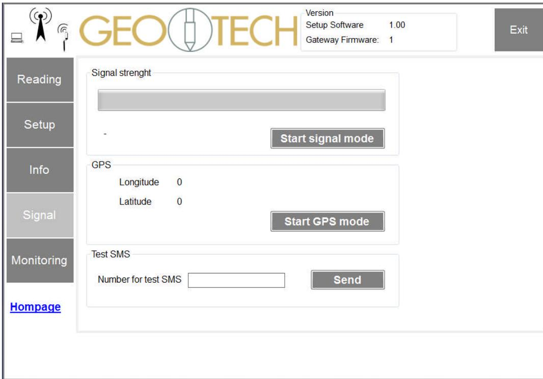
Use this function as help during installation. It will provide information about mobile phone network coverage and GPS position.
