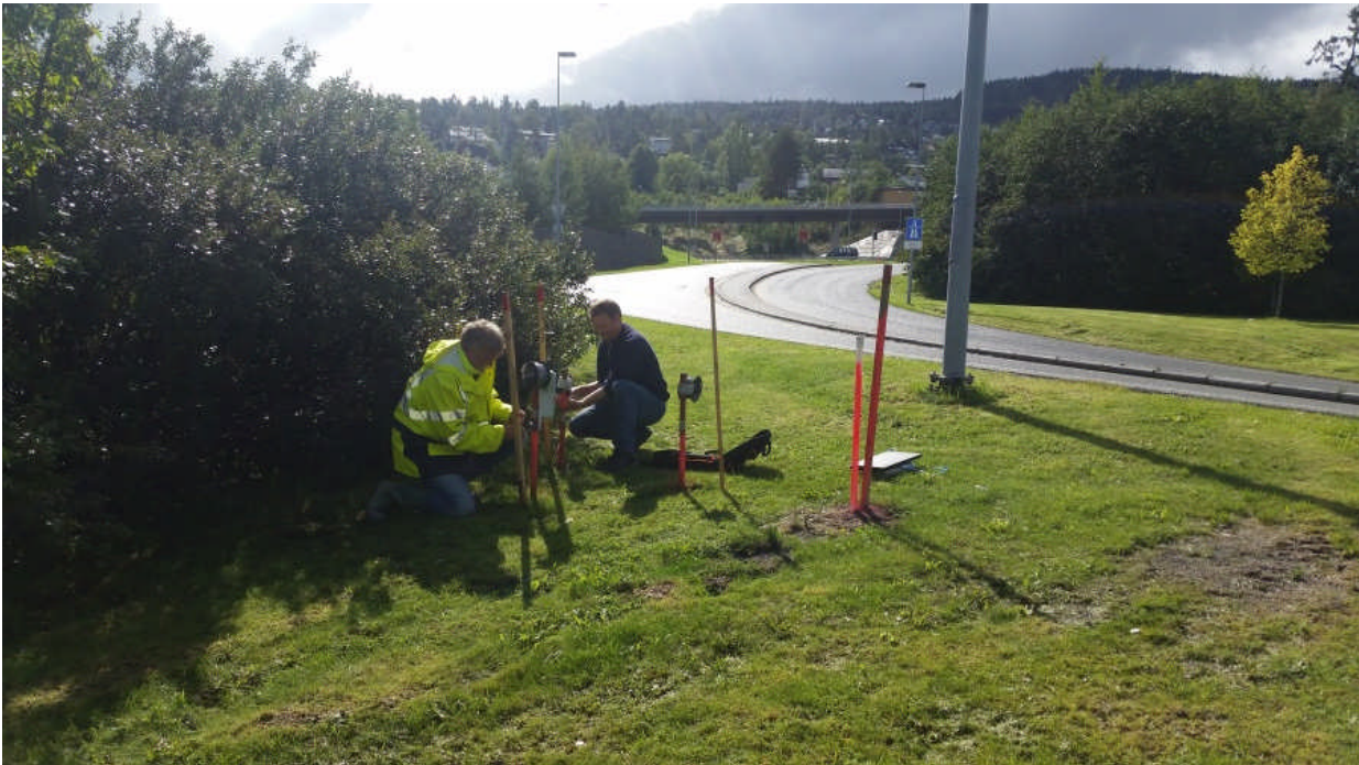
Fig. 1 – Remote read-out solution example: Monitoring of pore pressure in clay at different depths under a road. The gateway receives settings and sends logged data via the mobile phone network.
