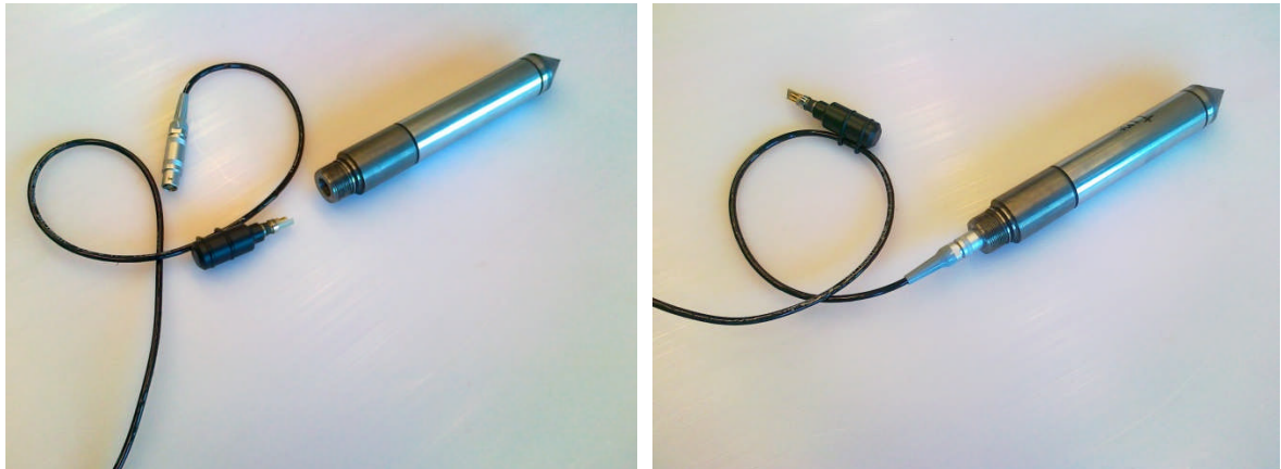
Fig. 22 – Synchronisation of the memory probe before test.
