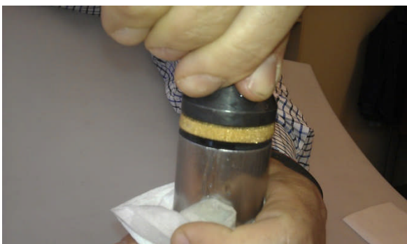
Fig. 19 – De-airing of CPT GEOTECH NOVA probe
