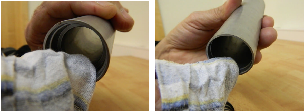
Fig. 28 – Cleaning the friction sleeve.
