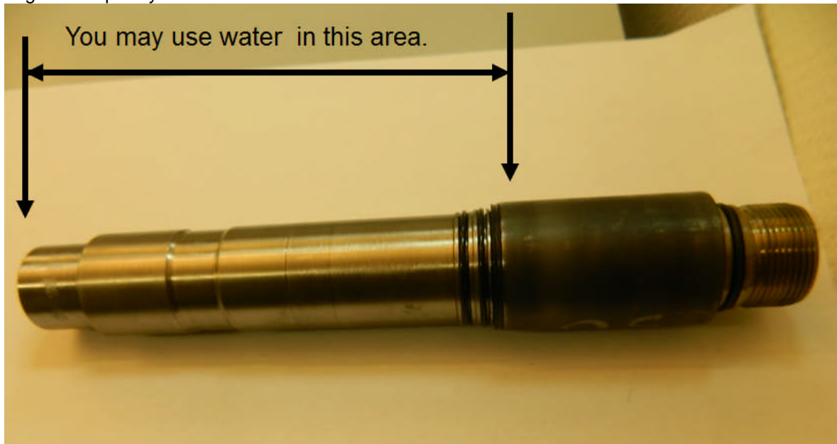
Fig. 29 – You may use water when cleaning the measuring body – but protect the contact area of the end piece from moist and water.
