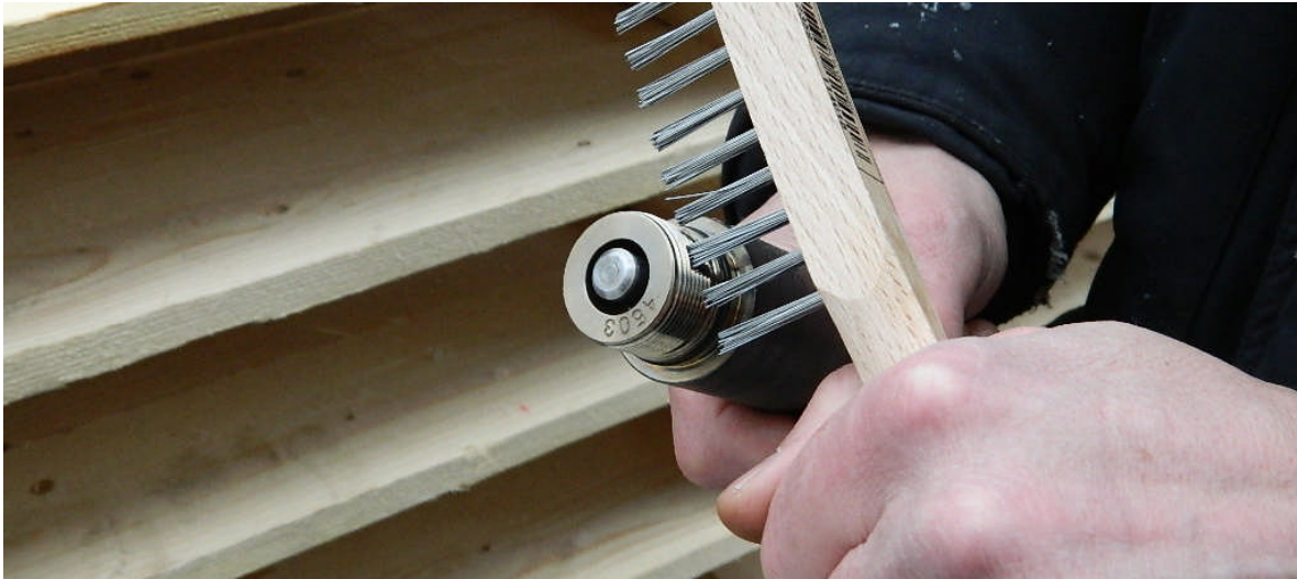
Fig. 30 – Cleaning the threads of the probe's en piece. Protect the contact area of the end piece from moist and water.
